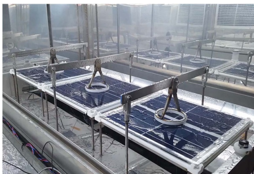
Figure 5. Combined accelerated test setup from NREL. [127] John Wiley & Sons. [© 2020 John Wiley & Sons, Ltd.].
