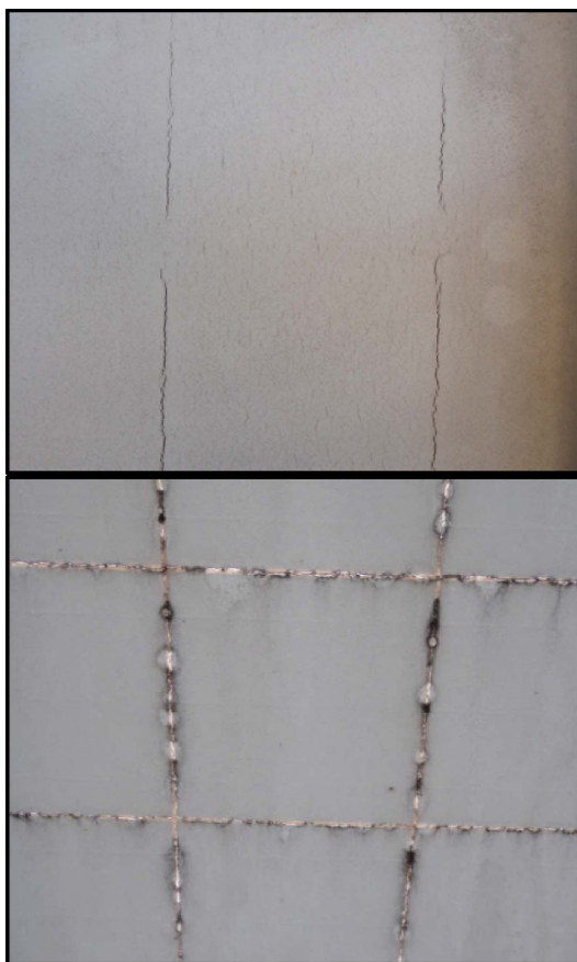
Figure 4. PA cracks. Longitudinal (top) and squared cracks (bottom) of PV modules with PA backsheets [9]. Reprinted from [9], Copyright (2019), with permission from Elsevier.
