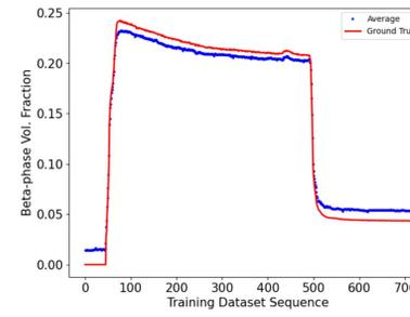
(left): Architecture of the CNN model trained 100 times. (right): CNN model's average predicted results. The red line represents the ground truth, while the blue plots depict the average predicted results. The MSE in this case is 3.47e-06
