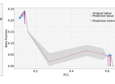
(left): Original vs. Predicted  $\beta$ -fraction with 95% prediction interval for test set using GPR. (right): Original vs. Predicted  $\beta$ -fraction with corresponding 95% prediction interval for PC1
