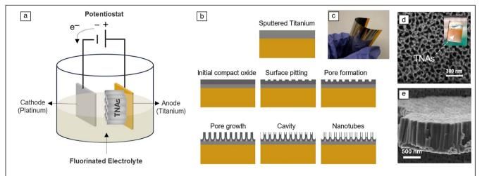
**Figure 2.** Schematic diagrams of (a) electrochemical anodization setup and (b) formation mechanism of titania nanotube arrays (TNAs) from Tisputtered polyimide substrate. (c) Photo of a flexed Ti-sputtered polyimide substrate. (d) Top-view and (e) cross-section scanning electron microscopy images of a freestanding piece of TNA grown on polyimide substrate. The inset in (d) shows the transparent as-anodized TNAs-on-polyimide substrate.
