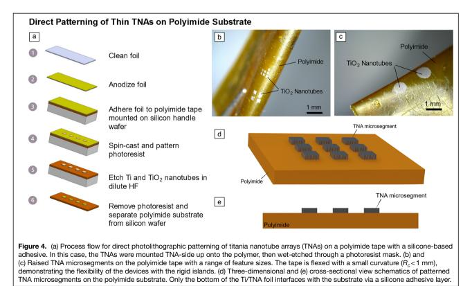
place at room temperature apart from a brief 60-s exposure to 110°C on a hot plate for photoresist processing. Therefore, this process can be applied to various substrate materials when accompanied by an adhesive layer.
